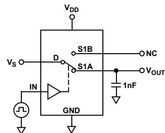
Figure 21. Charge Injection
