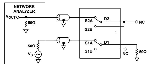
CHANNEL-TO-CHANNEL CROSSTALK =  $20 \log \frac{V_{OUT}}{VS}$
