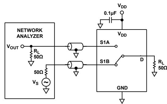
CHANNEL-TO-CHANNEL CROSSTALK =  $20 \log \frac{V_{OUT}}{VS}$
