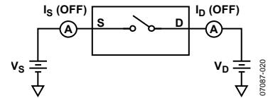
Figure 17. Off Leakage
