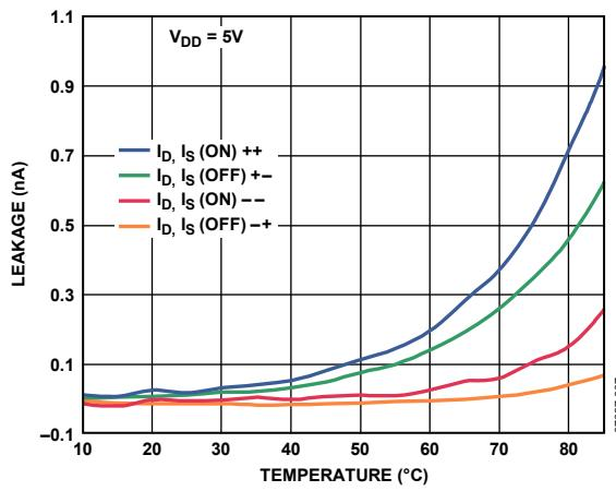
Figure 7. Leakage Current vs. Temperature,  $V_{DD}$  = 5 V
