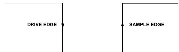
Figure 65. SPI Mode 3, SCLK Edges
