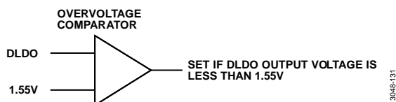
Figure 121. Digital LDO Monitor
