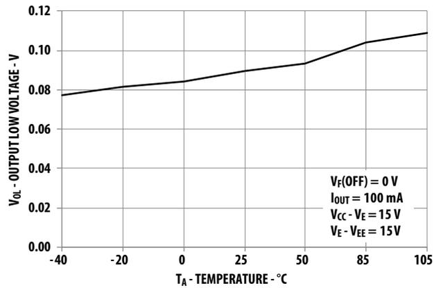
Figure 5  $I_{OL}$  vs. Temperature
