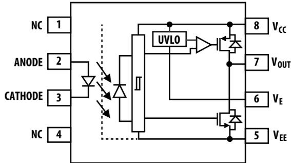
**Design Notes:** A 1- $\mu$ F bypass capacitor must be connected between pins  $V_{CC}$  and  $V_{EE}$ .
