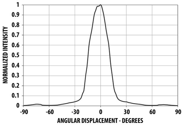
Figure 7. Representative Radiation pattern for 23° Viewing Angle Lamp
