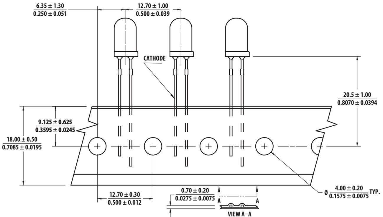
Note: The ammo-packs drawing is applicable for packaging option -DD & -ZZ and regardless standoff or non-standoff
