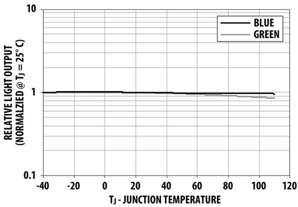
Figure 9. Relative Light Output vs Junction Temperature
