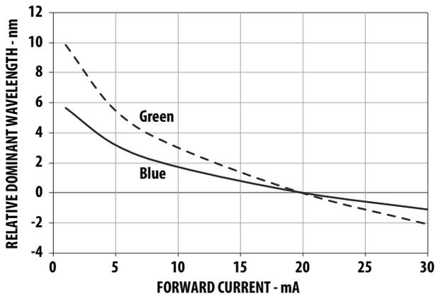
Figure 5. Relative Dominant Wavelength Shift vs Forward Current
