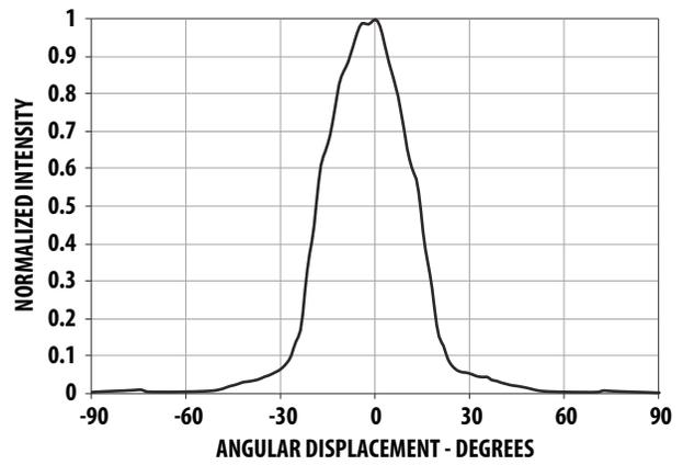
Figure 8. Representative Radiation pattern for 30° Viewing Angle Lamp
