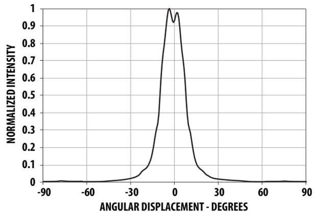
Figure 6. Representative Radiation pattern for 15° Viewing Angle Lamp
