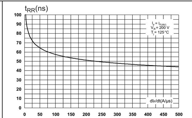
Figure 7. Reverse recovery charges versus  $di_F/dt$  (typical values, per diode)
