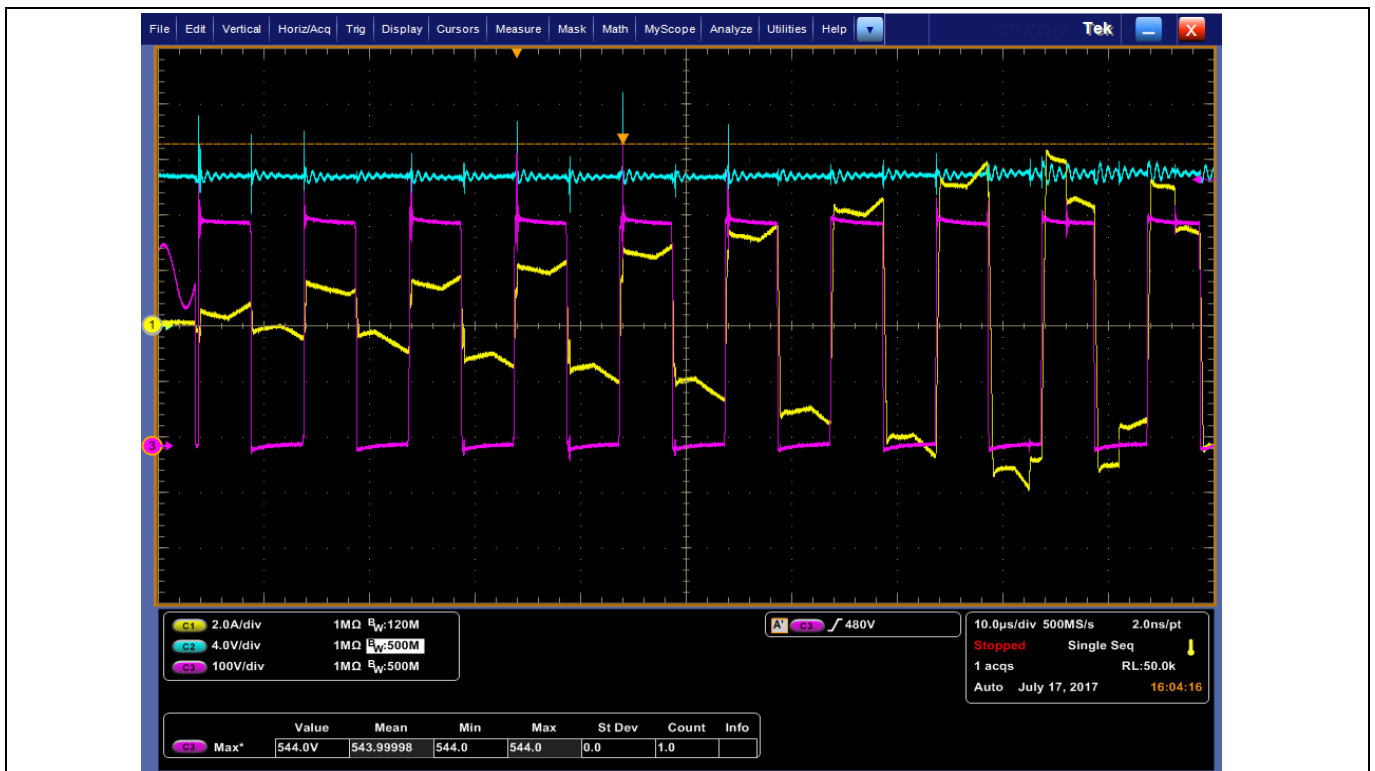
Figure 70 Short-circuit under full-load conditions at output. Primary current (yellow), MOSFET V_{DS} (purple), output voltage (blue).
