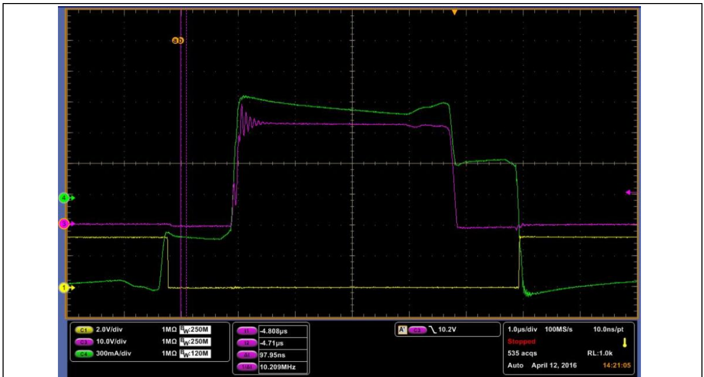
Figure 39 Synchronous MOSFET gate pulse (yellow), V_{DS} (purple) and primary current of the transformer (green)
