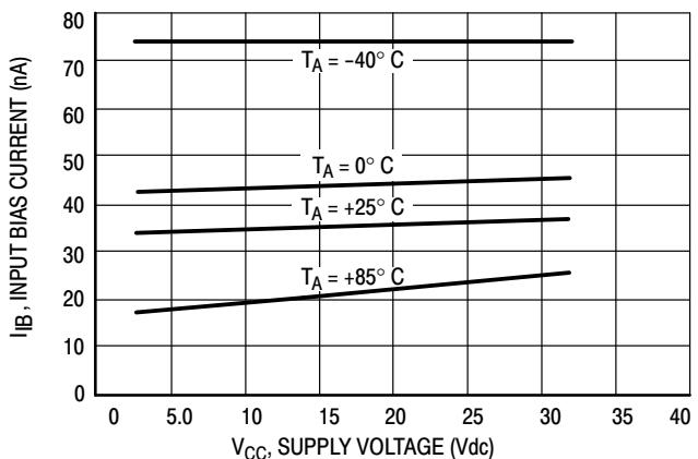
**Figure 3. Input Bias Current versus Power Supply Voltage**
