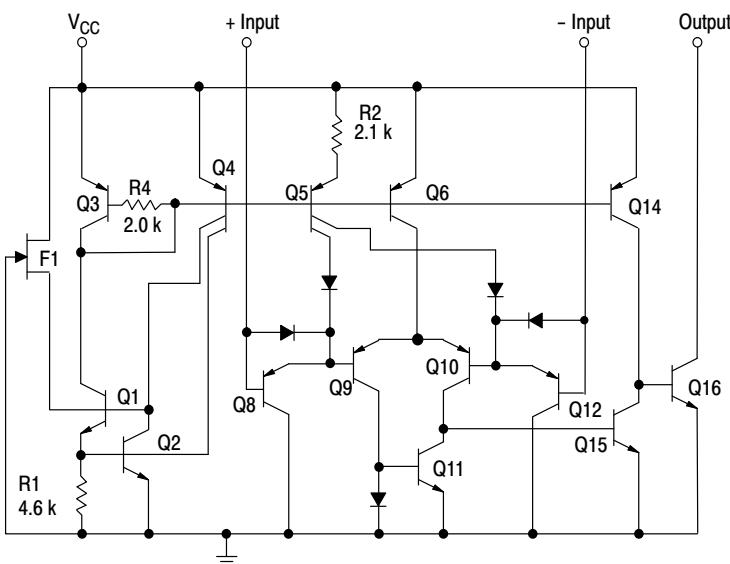
Figure 1. Representative Schematic Diagram
