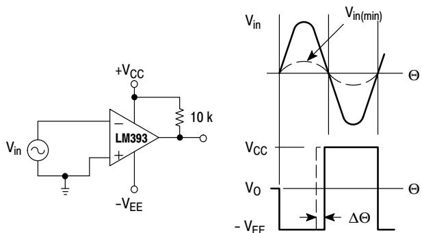
**Figure 9. Zero Crossing Detector
