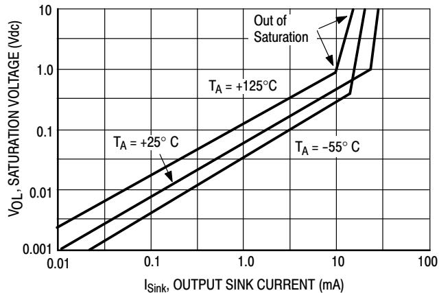
**Figure 4. Output Saturation Voltage versus Output Sink Current**
