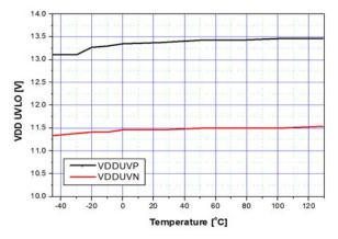
Figure 10. V<sub>DD</sub> UVLO vs. Temperature
