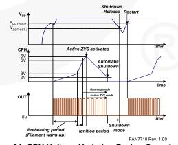
Figure 31. CPH Voltage Variation During Open-Lamp
