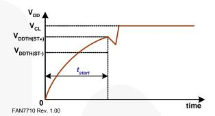
Figure 34. V<sub>DD</sub> Build-up
