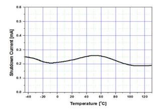
Figure 9. Shutdown Current vs. Temperature
