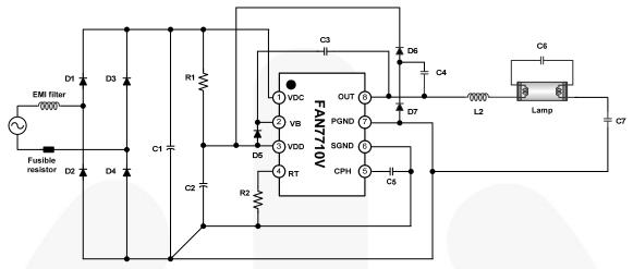
Figure 1. Typical Application Circuit for Compact Fluorescent Lamp
