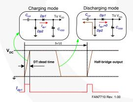
Figure 36. Charge Pump Operation
