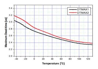
Figure 17. Maximum Dead Time vs. Temperature
