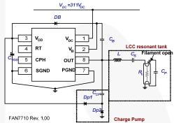
Figure 30. Current Flow When the Lamp is Open
