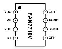
Figure 3. Pin Configuration (Top View)
