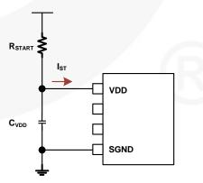
Figure 35. Equivalent Circuit During Startup
