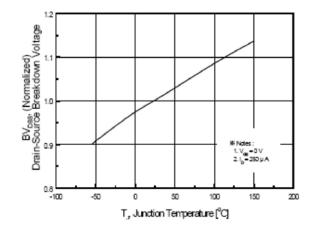
Figure 21. Breakdown Voltage Variation vs. Temperature
