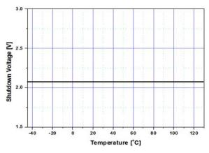
Figure 13. Shutdown Voltage vs. Temperature
