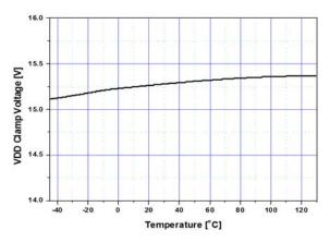
Figure 12. V<sub>DD</sub> Clamp Voltage vs. Temperature
