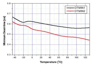
Figure 16. Minimum Dead Time vs. Temperature
