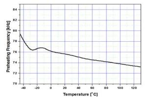
Figure 15. Preheating Frequency vs. Temperature
