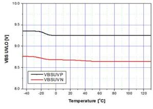
Figure 11. V<sub>BS</sub> UVLO vs. Temperature
