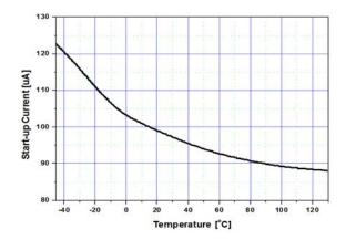
Figure 4. Startup Current vs. Temperature
