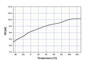
Figure 6. Ignition Current vs. Temperature
