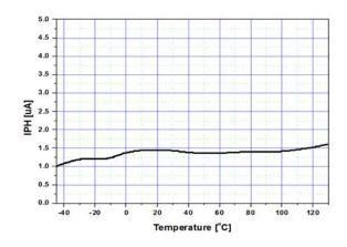
Figure 5. Preheating Current vs. Temperature
