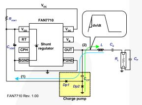
Figure 32. Local Power Supply for V<sub>DD</sub> Using a Charge-Pump Circuit
