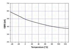
Figure 8. High-Side Quiescent Current vs. Temperature
