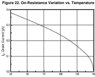
Figure 24. Maximum Drain-Current vs. Case Temperature
