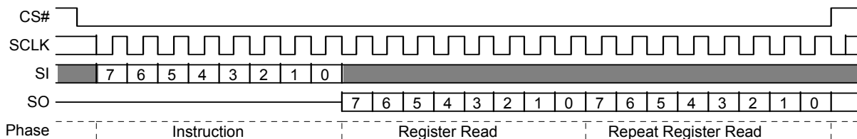
Figure 10.7 Read Configuration Register (RDCR) Command Sequence
