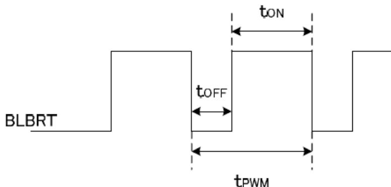
$t_{ON}, t_{OFF} = 50 \mu s$ .
