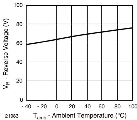
Fig. 3 - Reverse Voltage vs. Ambient Temperature
