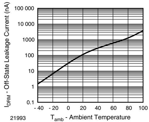
Fig. 5 - Off-State Leakage Current vs. Ambient Temperature
