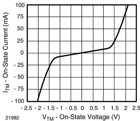
Fig. 4 - On-State Current vs. On-State Voltage
