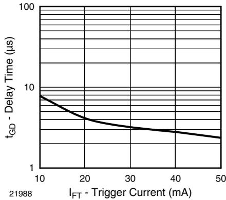
Fig. 9 - Trigger Current vs. Delay Time
