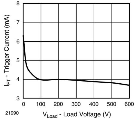
Fig. 11 - Trigger Current vs. Load Voltage
