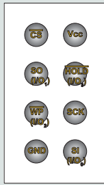
Figure 1-3. 8-ball WLCSP (Bottom View)
