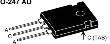
A = Anode, C = Cathode, TAB = Cathode
