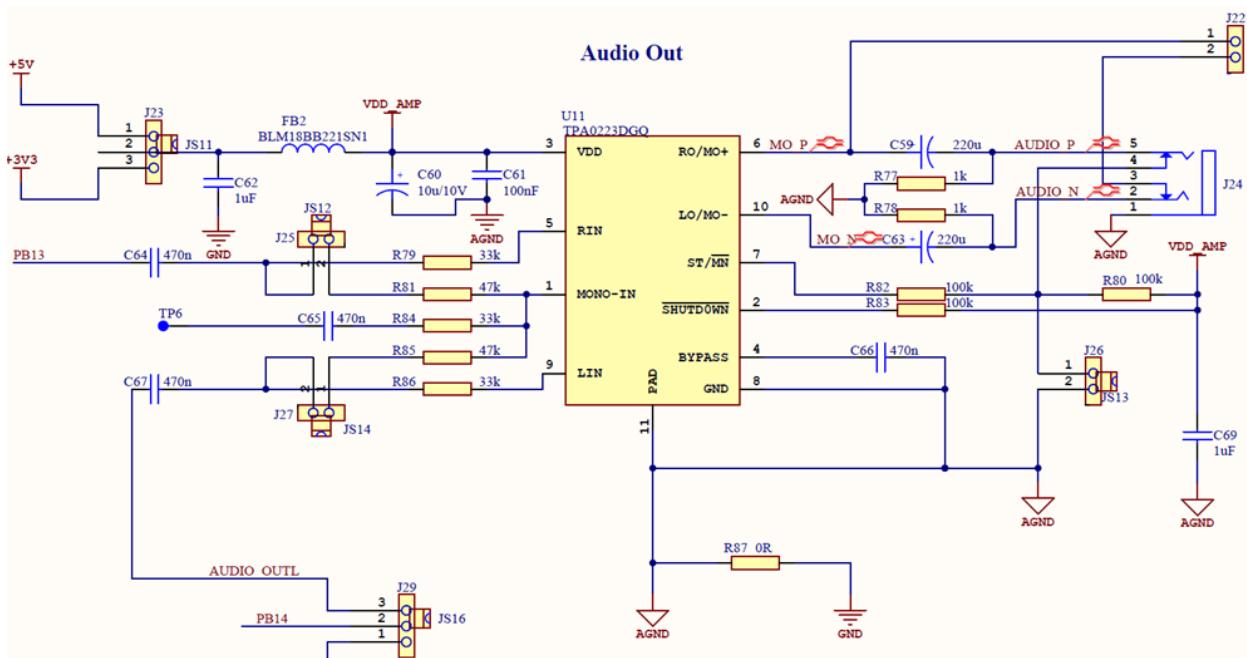
Using a readily available 1/8-in. (3.5mm) stereo headphone jack, the control switch (pin4 and pin5 in J24) is closed when no plug is inserted. When closed, a  $100k\Omega/1k\Omega$  divider pulls the ST/MN input low. When a jack plug is inserted, the  $1k\Omega$  resistor is disconnected and the ST/MN input is pulled high. The mono speaker (J22 connector) is also physically disconnected from the RO/MO+ output so that no sound is heard from the speaker while the headphones are inserted.
