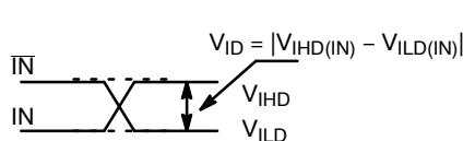
**Figure 6. Differential Inputs Driven Differentially**
