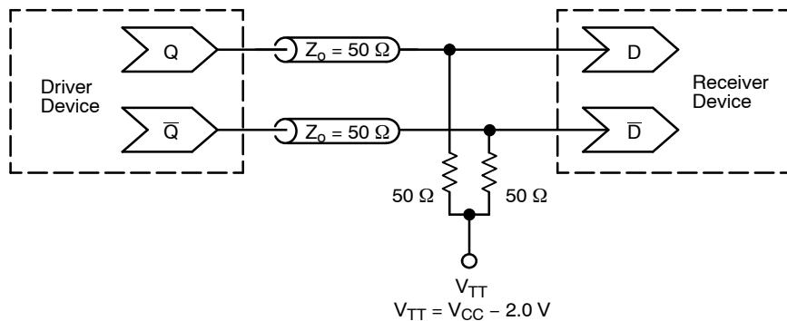
**Figure 10. Typical Termination for Output Driver and Device Evaluation
