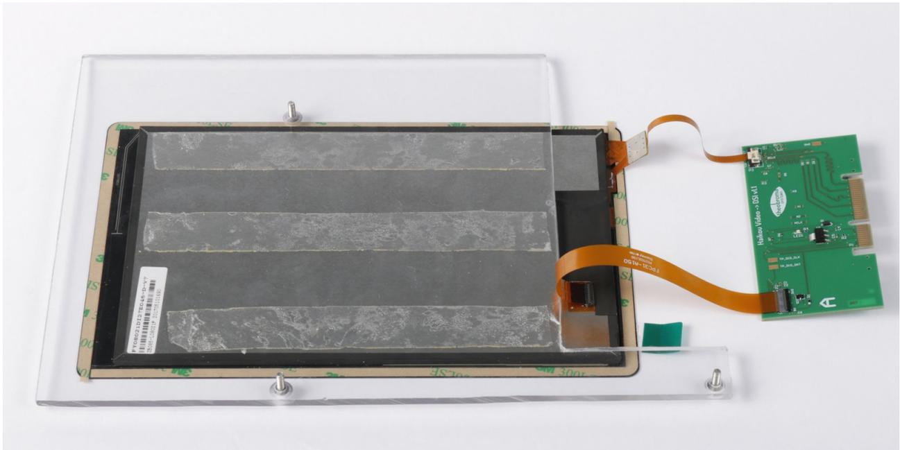
Fig. 1.2: Flat-flex cabling
