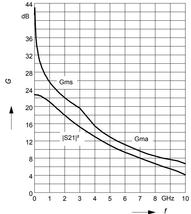
**Power gain  $G_{ma}, G_{ms} = f(V_{CE})$**
