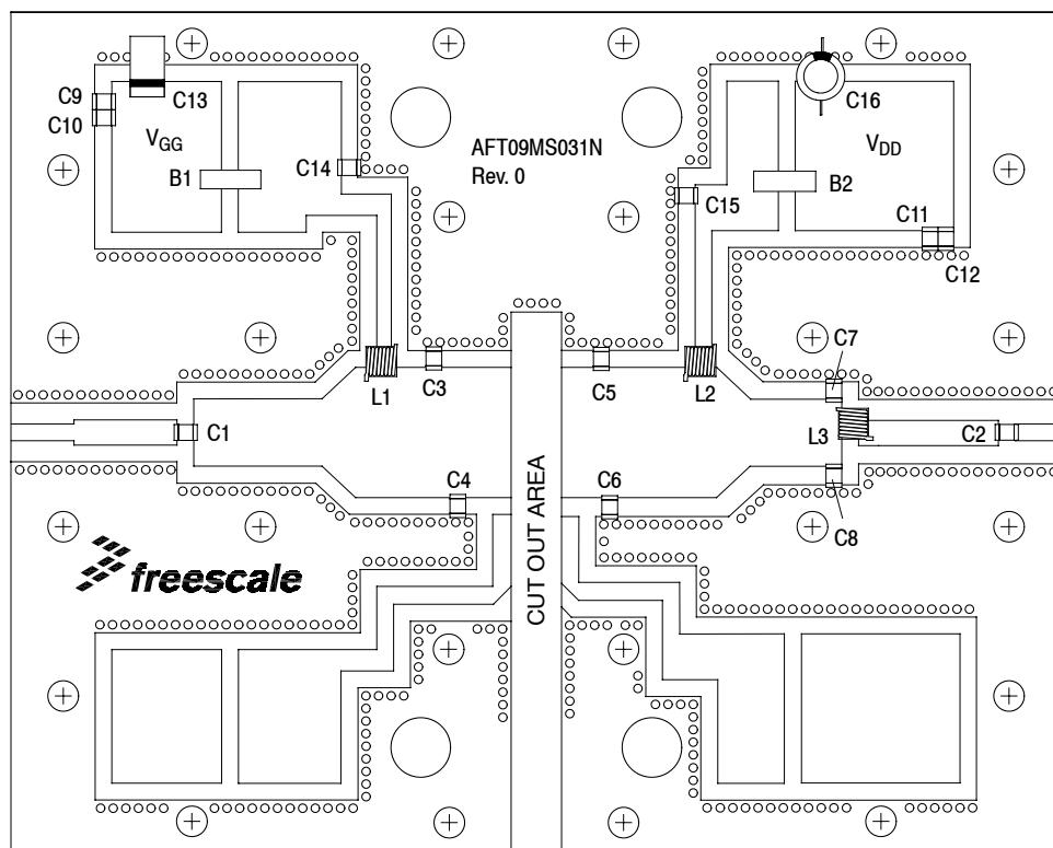
Figure 5. AFT09MS031NR1 Narrowband Test Circuit Component Layout — 870 MHz
