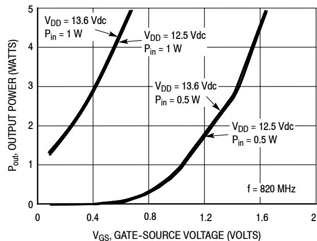
**Figure 14. CW Output Power versus Gate-Source Voltage**
