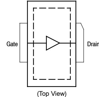
Note: The backside of the package is the source terminal for the transistor.
