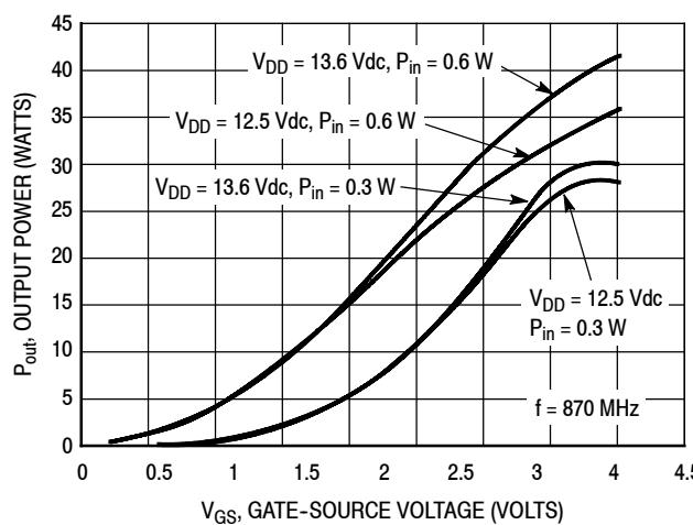
Figure 7. CW Output Power versus Gate-Source Voltage
