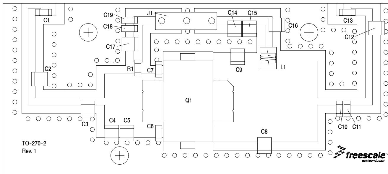
Figure 10. AFT09MS031NR1 Broadband Reference Circuit Component Layout — 760-870 MHz
