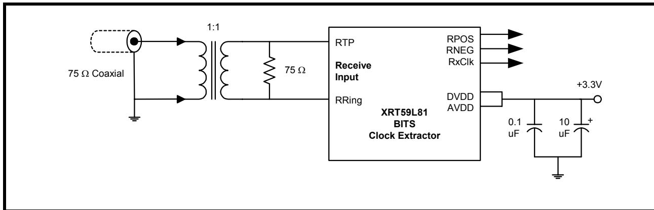
FIGURE 13. T1 APPLICATION FOR TWISTED PAIR INTERFACE
