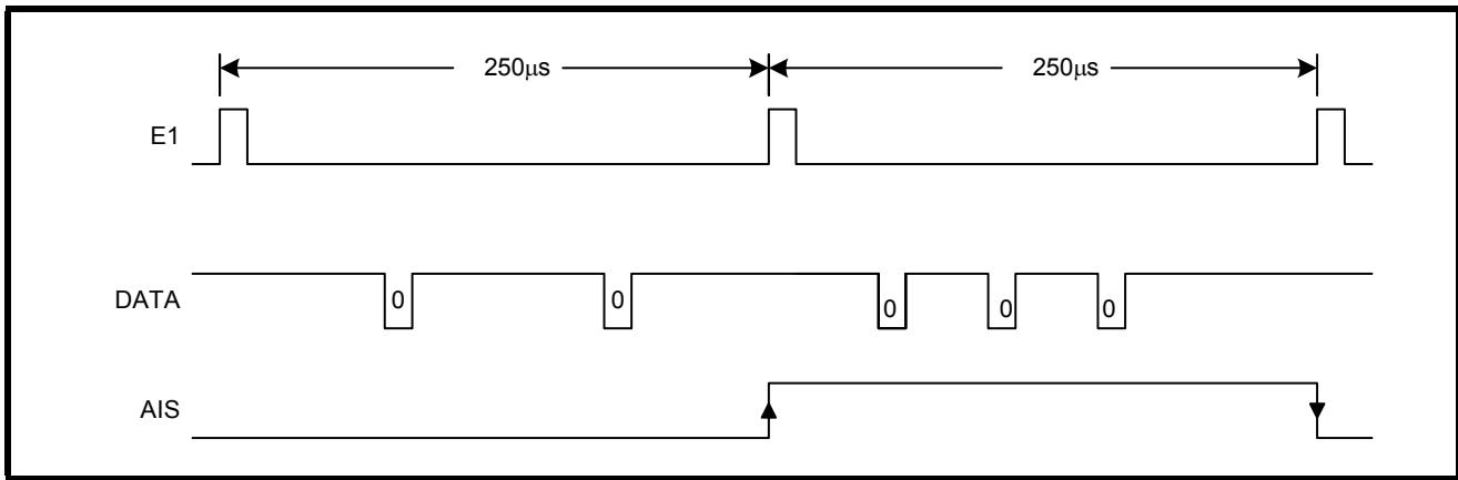
In T1 mode, AIS is detected if the received input signal has 4 or less Zero's in a sequence of 4632 bits (3ms) and AIS is cleared when 5 or more Zero's are detected in the subsequent 4632 bits (3 ms) time-frame. Figure 10 shows the AIS timing for T1 mode.
