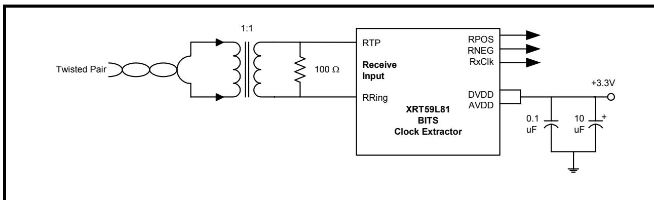
**FIGURE 14. 64KBPS APPLICATION FOR TWISTED PAIR**
