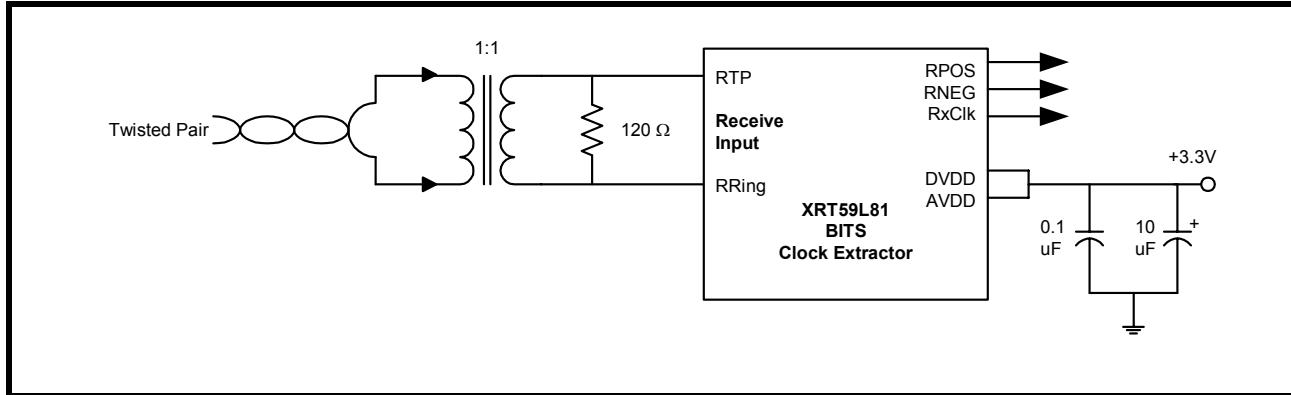
FIGURE 12. CEPT APPLICATION FOR COAXIAL INTERFACE
