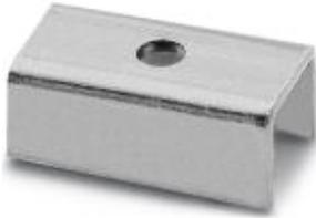
Flat bracket, for fixing DIN rails 15 mm above the mounting surface, the fixing hole has a diameter of 6.5 mm
