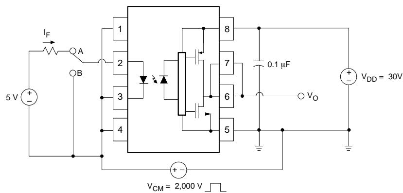
Figure 28. CMR Test Circuit and Waveforms
