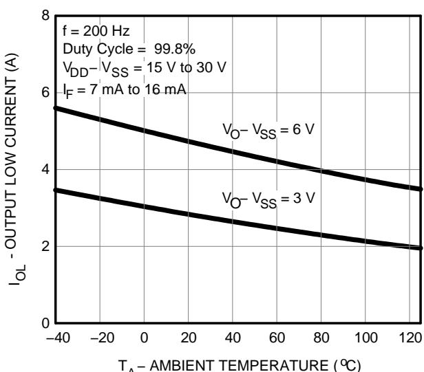
**Figure 6. Output Low Current vs. Ambient Temperature**
