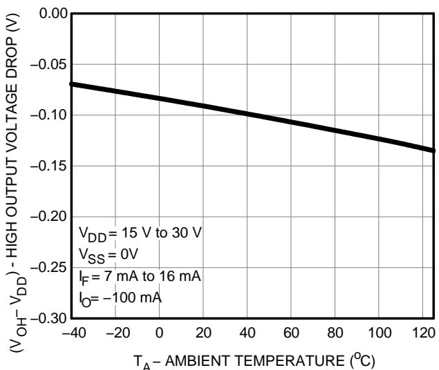
**Figure 2. Output High Voltage Drop vs. Ambient Temperature**
