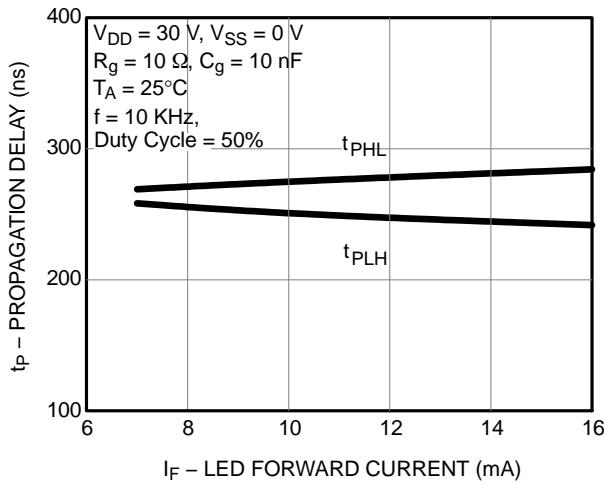
Figure 11. Propagation Delay vs. LED Forward Current
