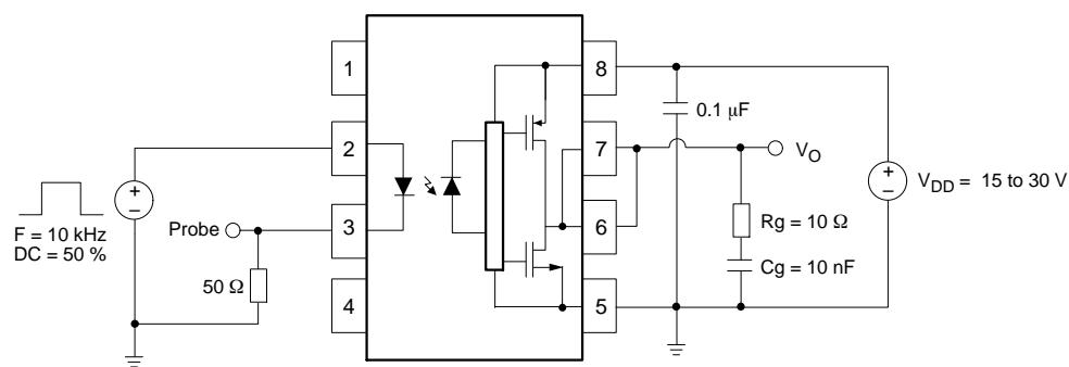
Figure 27.  $t_{PHL}$ ,  $t_{PLH}$ ,  $t_R$  and  $t_F$  Test Circuit and Waveforms
