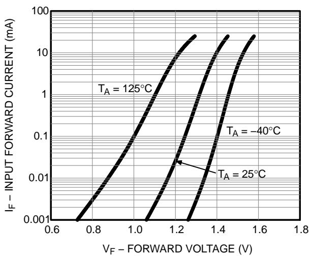
Figure 16. Input Forward Current vs. Forward Voltage
