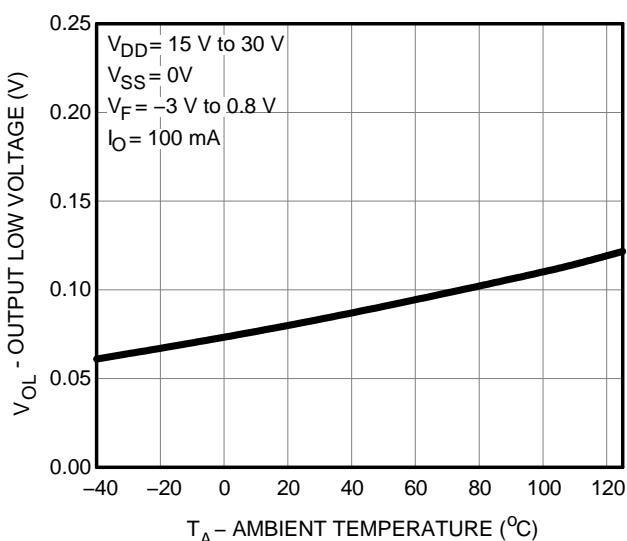
**Figure 5. Output Low Voltage vs. Ambient Temperature**
