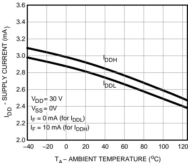
**Figure 7. Supply Current vs. Ambient Temperature**
