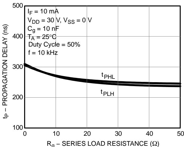
Figure 13. Propagation Delay vs. Series Load Resistance
