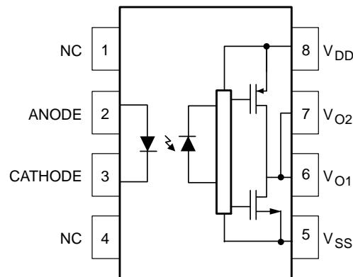
Note: A 0.1  $\mu\text{F}$  bypass capacitor must be connected between pins 5 and 8.
