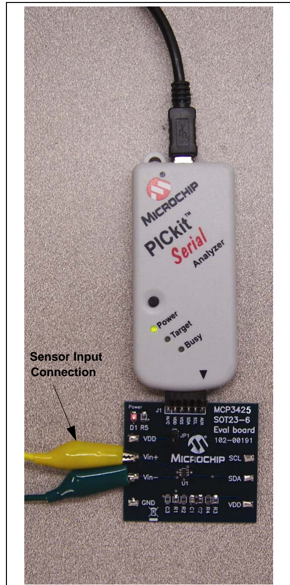
FIGURE 7-2: Setup for the MCP3425 Evaluation Board with PICKit™ Serial Analyzer.
