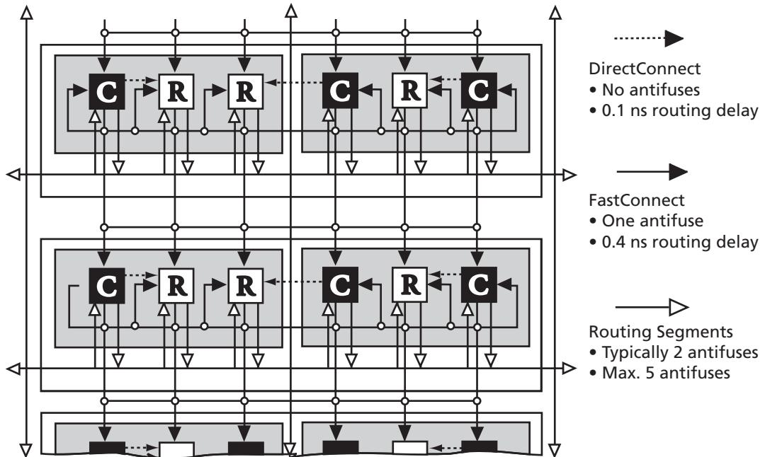
Figure 1-6 • DirectConnect and FastConnect for Type 2 SuperClusters
