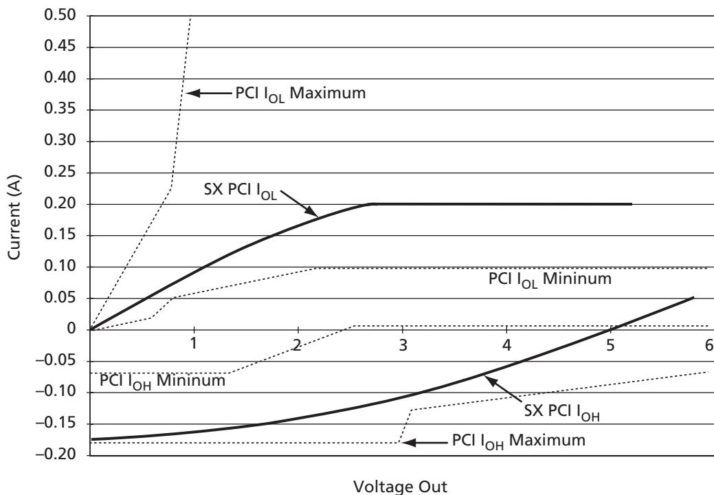
Figure 1-9 • 5.0 V PCI Curve for A54SX16P Device
