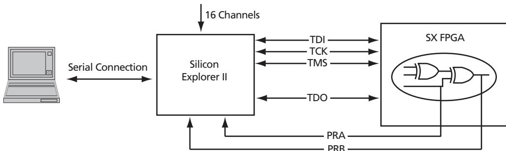
Figure 1-8 • Probe Setup
