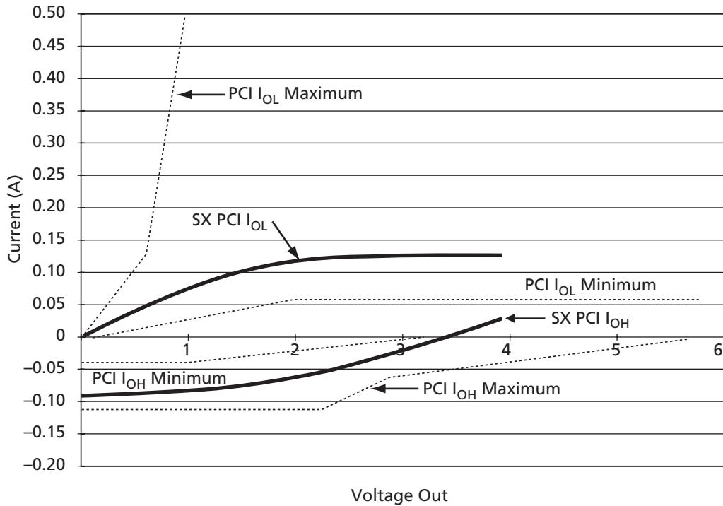
Figure 1-10 • 3.3 V PCI Curve for A54SX16P Device
