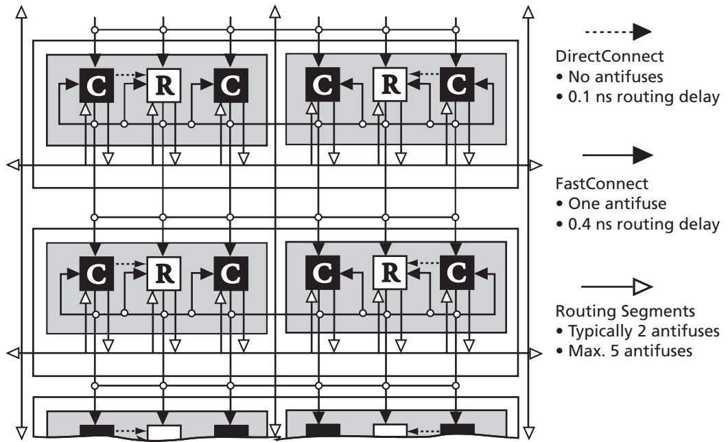
Figure 1-5 • DirectConnect and FastConnect for Type 1 SuperClusters
