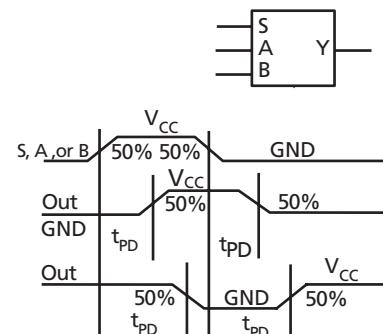
Figure 1-16 • C-Cell Delays
