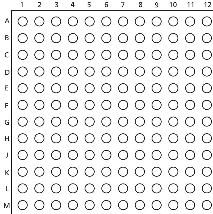
Figure 2-8 • 144-Pin FBGA (Top View)
