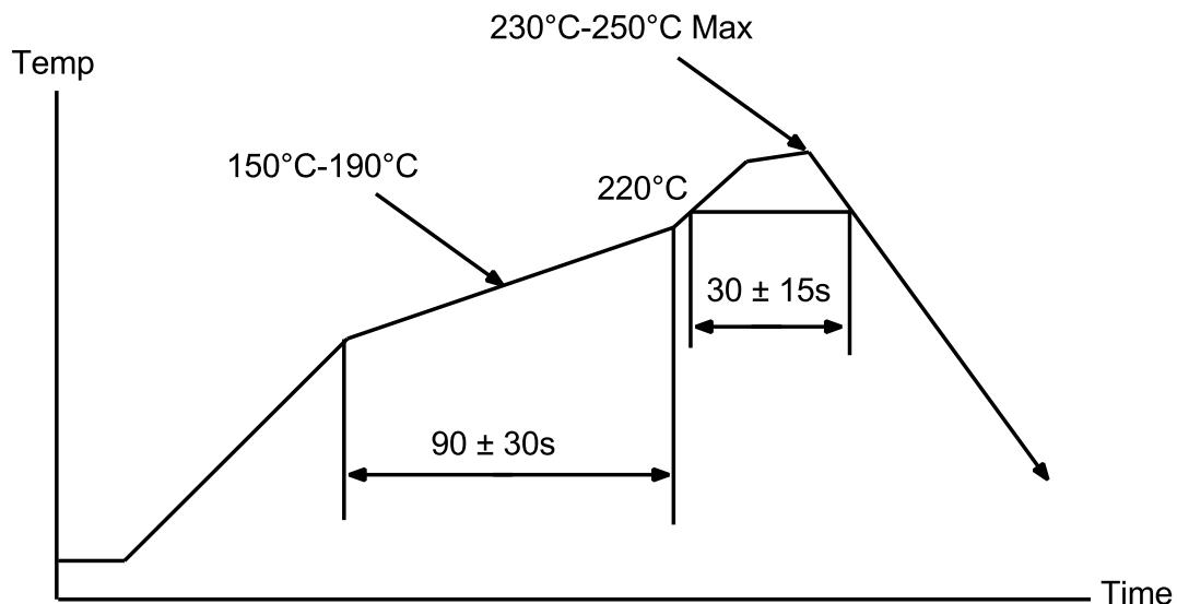
Figure 19 - Reflow Profile for Lead Free Solder
