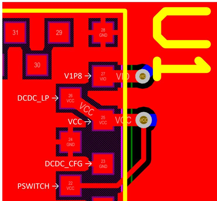
Figure 7 - PCB: Boost Mode Suggested Layout
