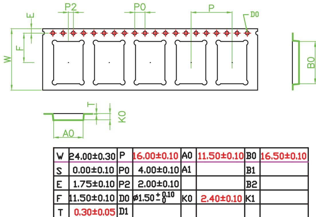
Figure 20 - Carrier Tape Dimension
