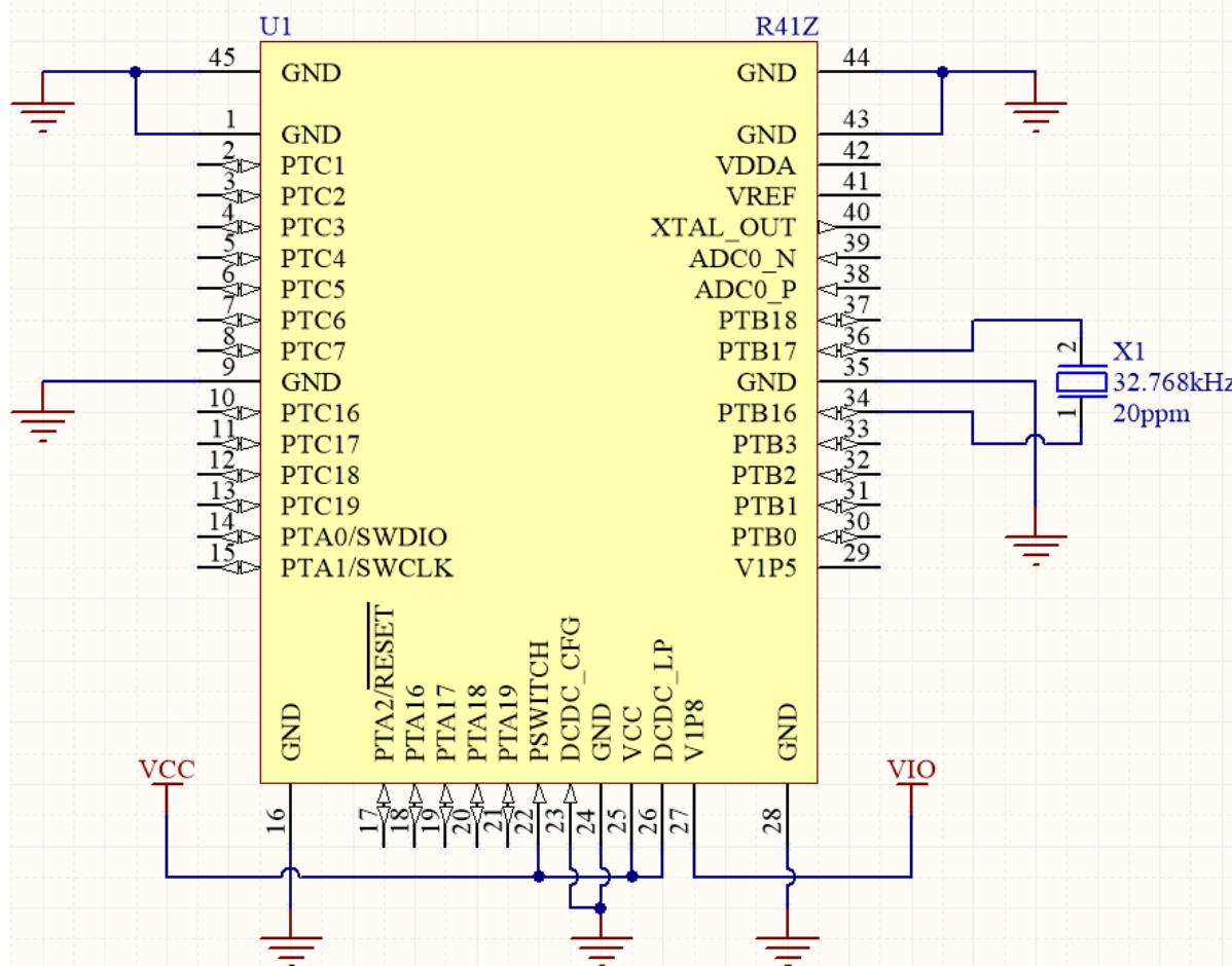
*Figure 6 - Schematic: DCDC Boost Mode Example*
