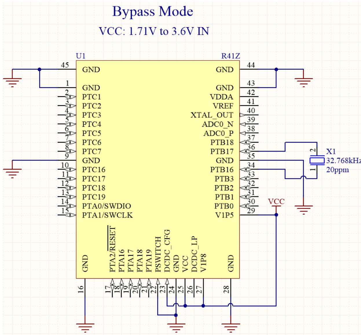
Figure 3 - Schematic: DCDC Bypass Mode Example
