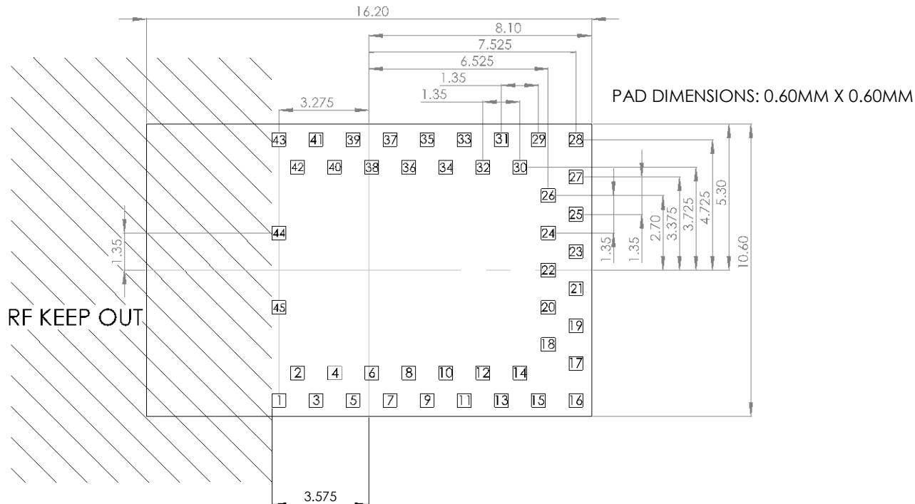
*Figure 11 - R41Z Pad Layout (Top View)*
