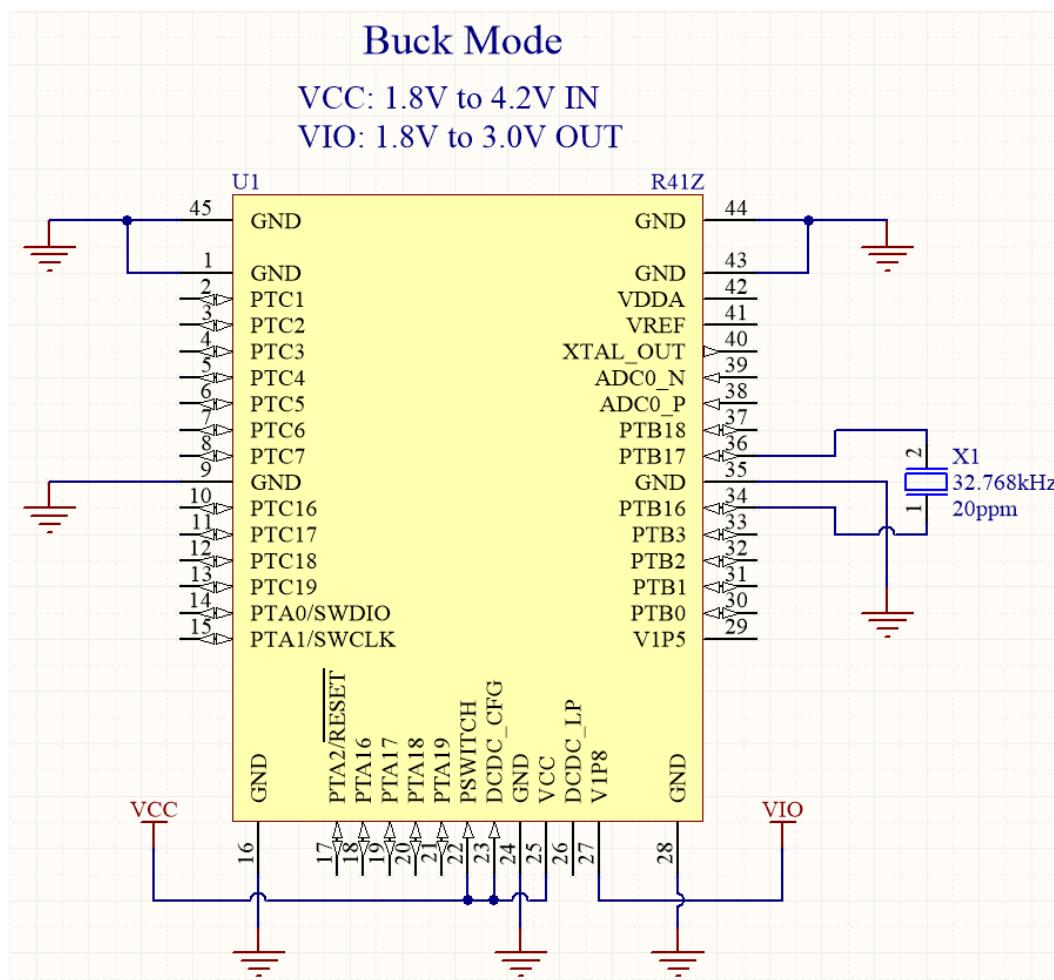
Figure 4 - Schematic: DCDC Buck Mode Example
