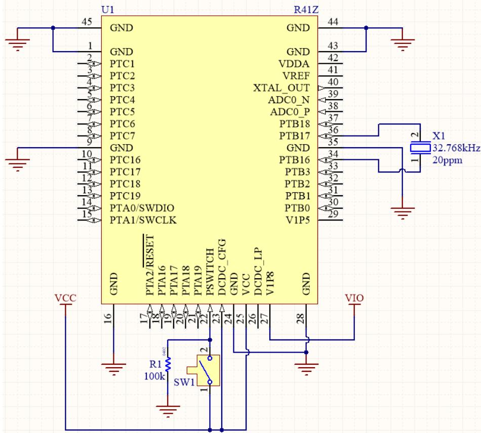
Figure 5 - Schematic: DCDC Buck Mode PSWITCH Example
