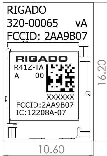
*Figure 12 - R41Z Module Marking - RevA*
