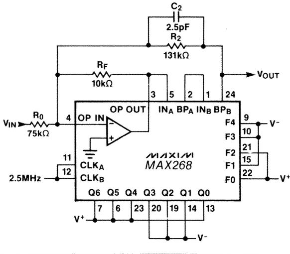
Figure 19. 4th-Order 50kHz Chebyshev Bandpass Using Multiple Feedback
