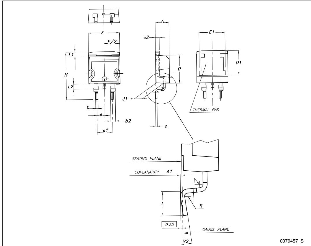
**Figure 20.** D<sup>2</sup>PAK footprint<sup>(a)</sup>
