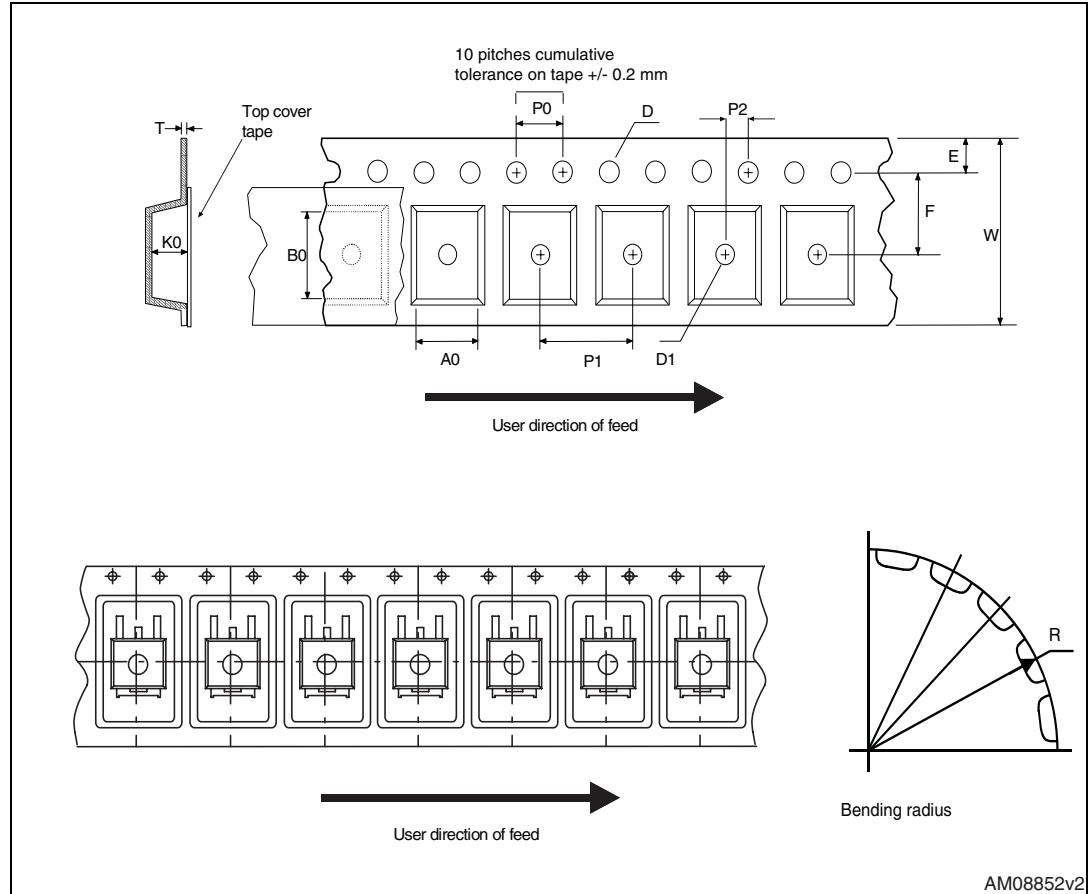
**Figure 24. Reel for D<sup>2</sup>PAK (TO-263) and DPAK (TO-252)**
