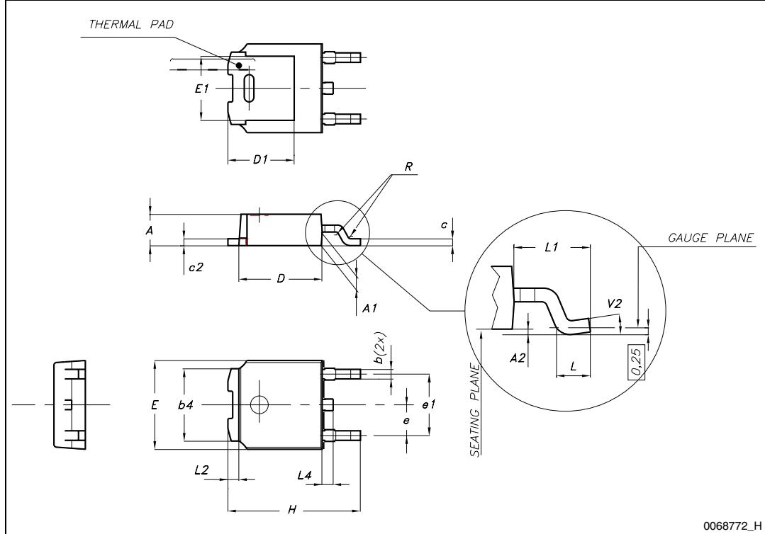
**Figure 22.** DPAK footprint(b)
