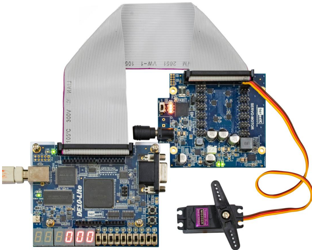
Figure 3-4 Demo Setup for DE10-Lite
