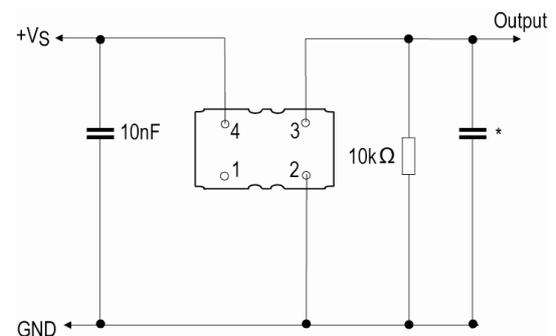
\*10k  $\Omega$  // 10pF (Clipped Sinewave), inclusive of probe and jig capacitance.
