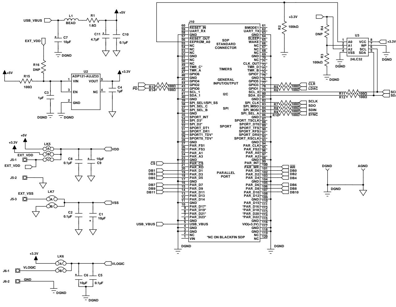
Figure 8. EVAL-MBnanoDAC-SDZ Motherboard SDP-B Connector and Power Supply
