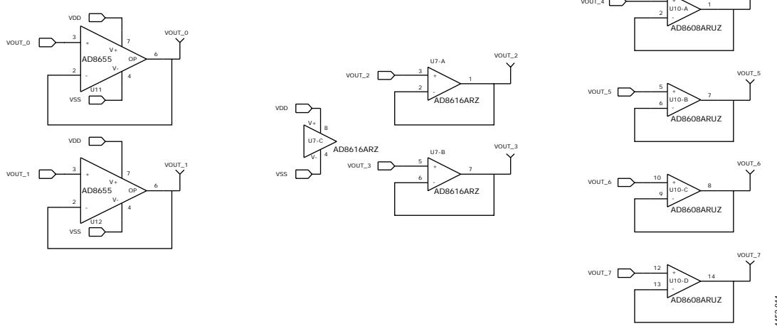
Figure 11. EVAL-MBnanoDAC-SDZ Motherboard Output Amplifier Circuit
