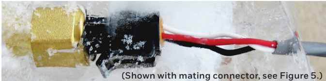
Figure 2. PX3 Series External Freeze/Thaw Resistance
