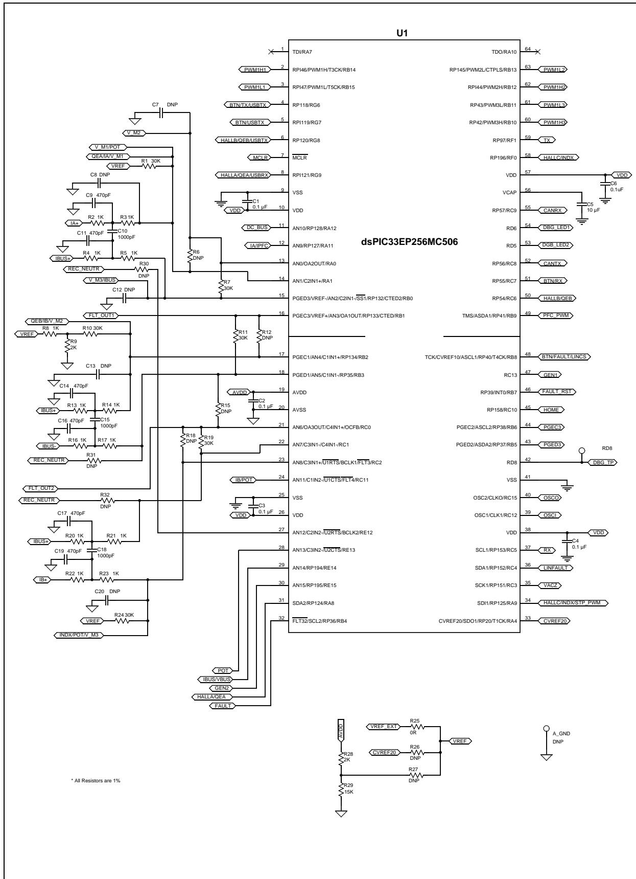
In the schematic shown in [Figure 3](#), resistors R25, R26 and R27 are used to choose the reference voltage (VREF) from motor control board (VREF\_EXT) or device internal reference (CVREF20) or a simple voltage divider (R28-R29), respectively. By default, the PIM is configured to source the reference voltage from the motor control board.
