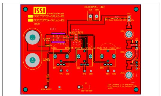
Figure 4: Board PCB Layout- Top Layer
