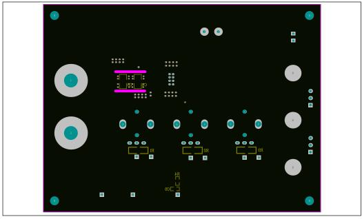
Figure 5: Board Component Placement Guide - Bottom Layer
