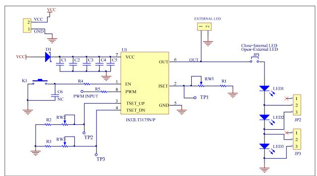
Figure 2: IS32LT3175N/P Application Schematic
