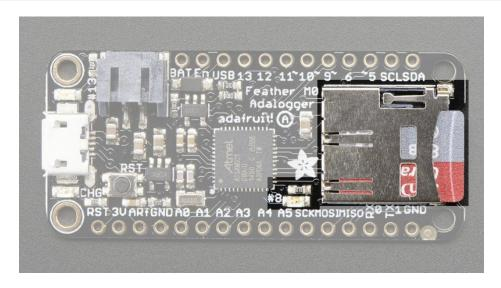
Since not all pins can be brought out to breakouts, due to the small size of the Feather, we use these to control the SD card!
