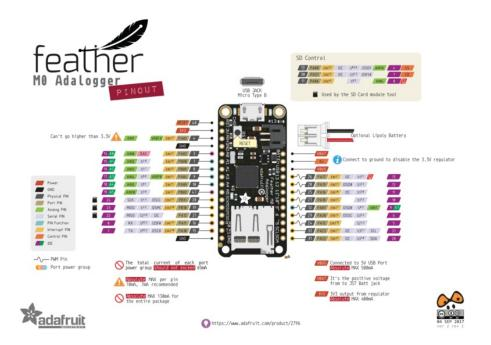
Note AREF in the diagram should be marked PA03 not PA02
