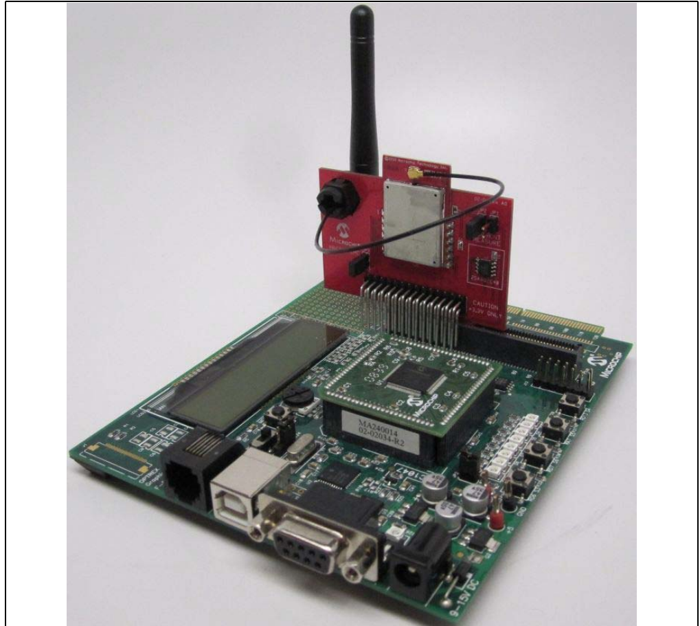
FIGURE 2-2: MRF24J40MC PICtail™/PICtail PLUS DAUGHTER BOARD PLUGGED INTO EXPLORER 16 DEVELOPMENT BOARD
