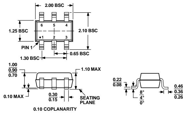
Figure 24. 6-Lead SC70 Package
