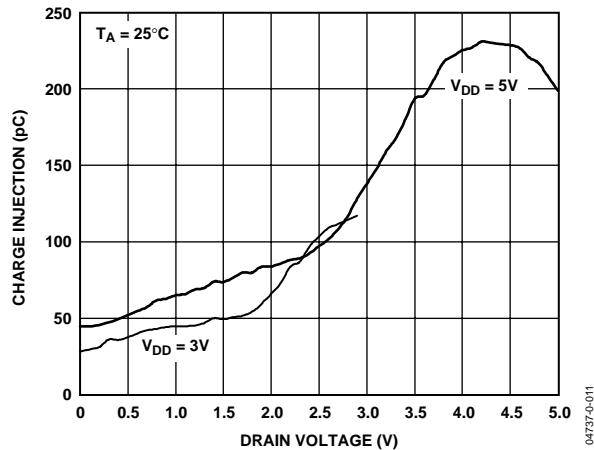
Figure 9. Charge Injection
