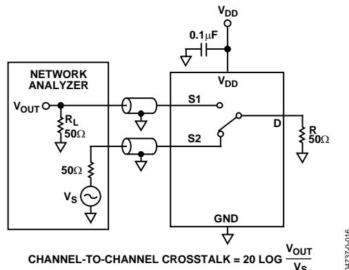
Figure 22. Channel-to-Channel Crosstalk
