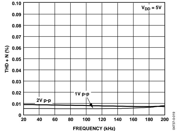
Figure 14. Total Harmonic Distortion + Noise
