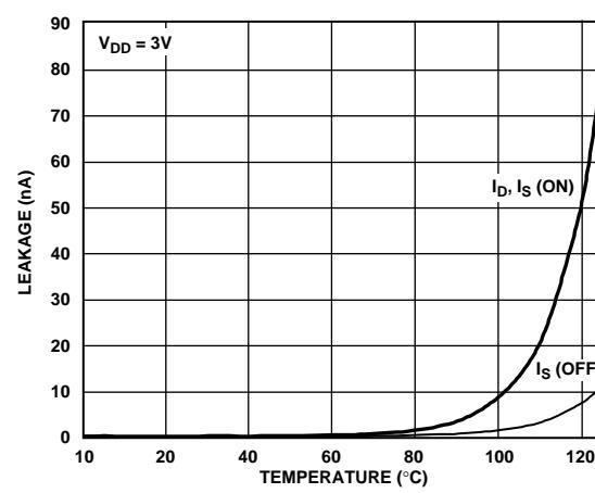
Figure 8. Leakage Currents vs. Temperature,  $V_{DD} = 3\text{ V}$
