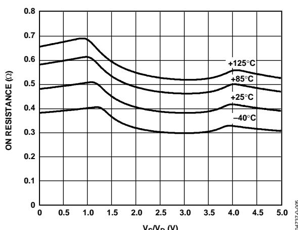
Figure 5. On-Resistance vs. Temperature,  $V_{DD} = 5 V$
