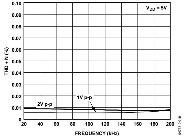
Figure 14. Total Harmonic Distortion + Noise
