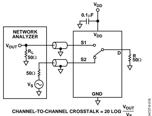
Figure 22. Channel-to-Channel Crosstalk
