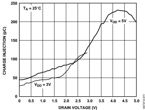
Figure 9. Charge Injection
