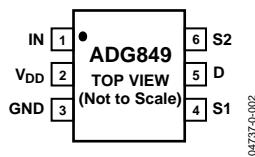
Figure 2. Pin Configuration
