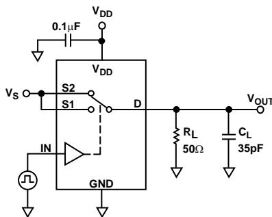
Figure 19. Break-Before-Make Time Delay,  $t_{BBM}$
