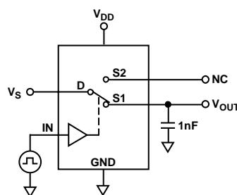
Figure 20. Charge Injection
