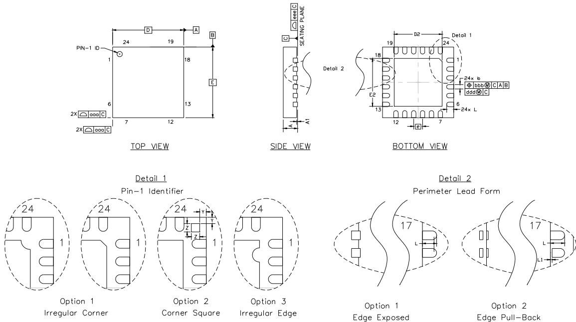
Figure 5.1. QFN-24 Package Drawing
