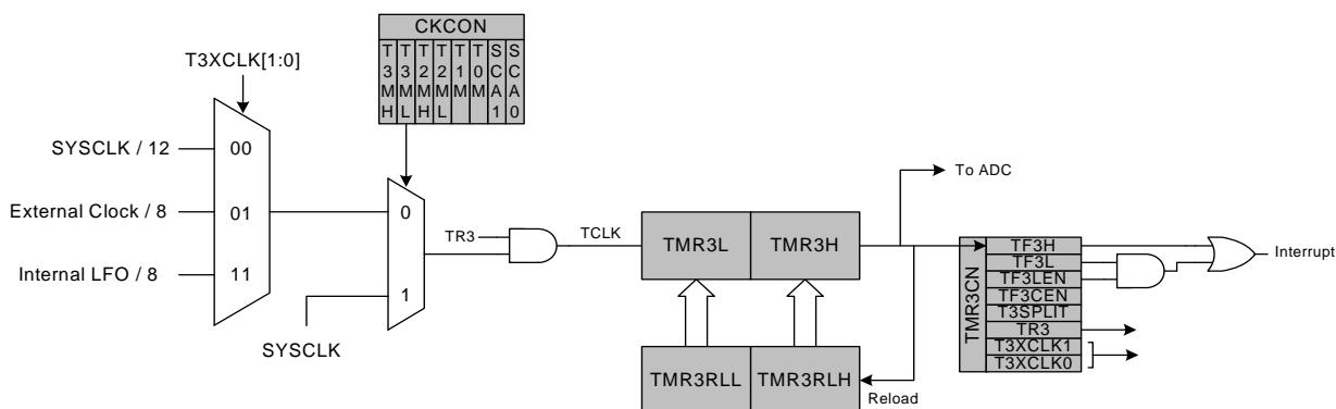
Figure 24.7. Timer 3 16-Bit Mode Block Diagram
