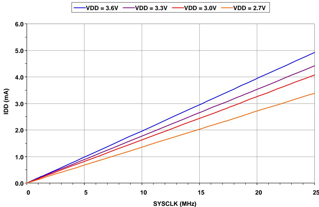
Figure 6.2. Idle Mode Digital Supply Current vs. Frequency
