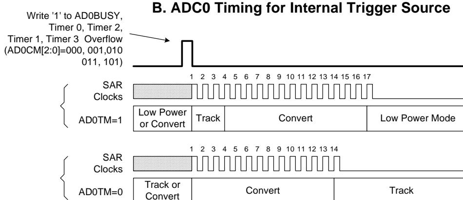
**Figure 7.2. 10-Bit ADC Track and Conversion Example Timing**
