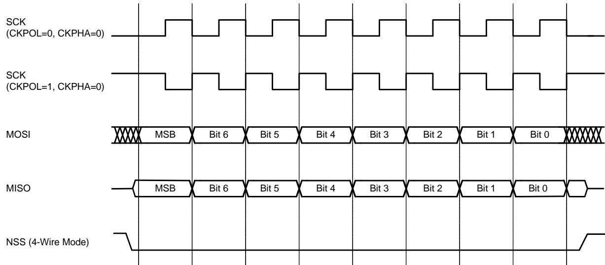
Figure 23.6. Slave Mode Data/Clock Timing (CKPHA = 0)
