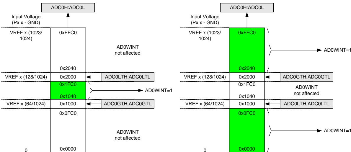
**Figure 7.5. ADC Window Compare Example: Left-Justified Single-Ended Data**
