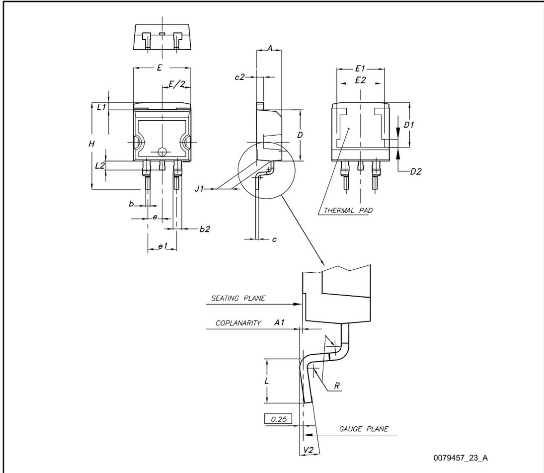
Table 9: D<sup>2</sup>PAK (TO-263) type A package mechanical data
