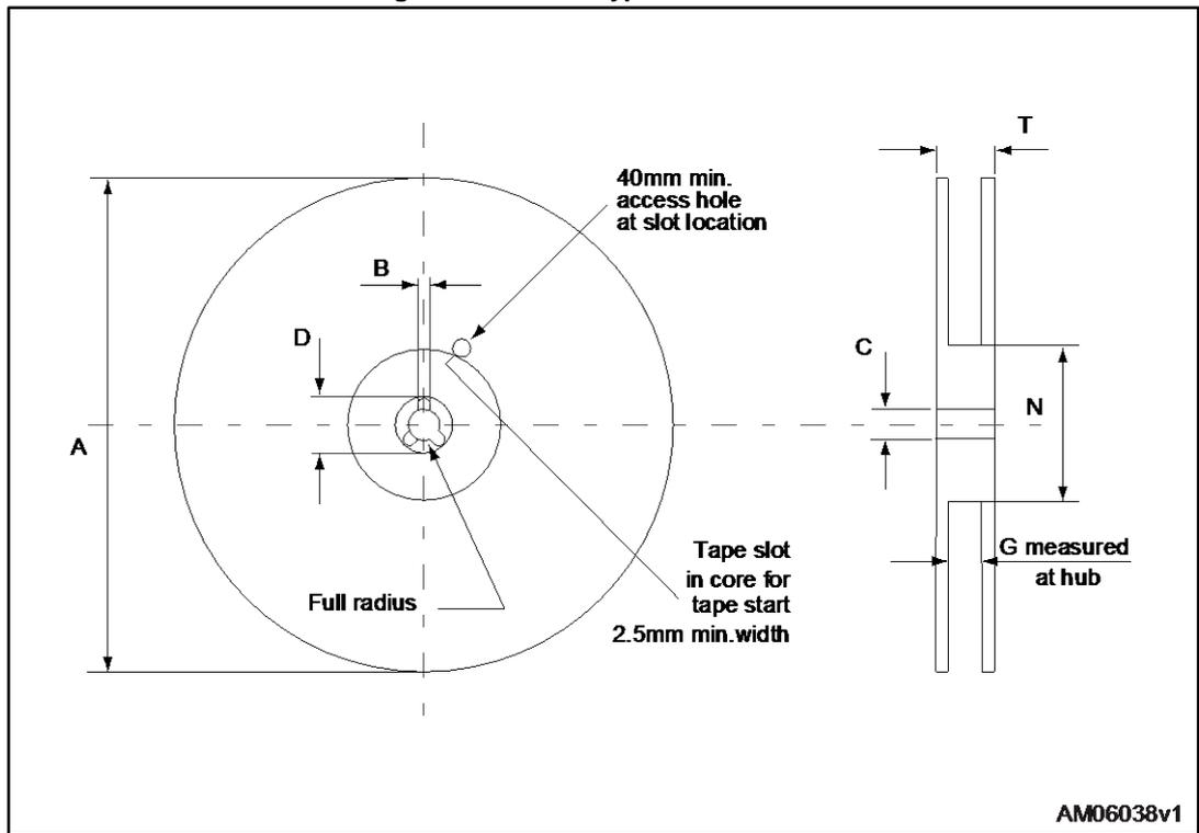
Table 11: D<sup>2</sup>PAK type A tape and reel mechanical data
