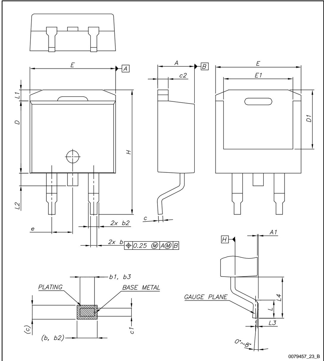
Table 10: D<sup>2</sup>PAK (TO-263) type B mechanical data
