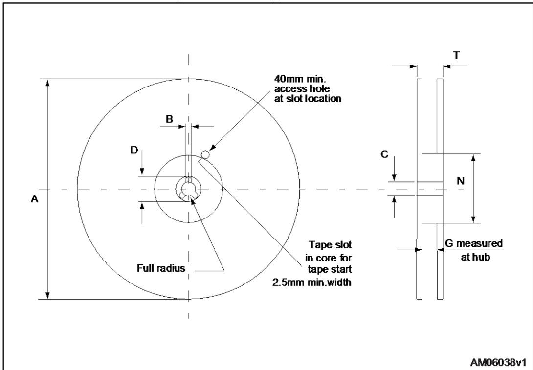
Table 12: D<sup>2</sup>PAK type B reel mechanical data
