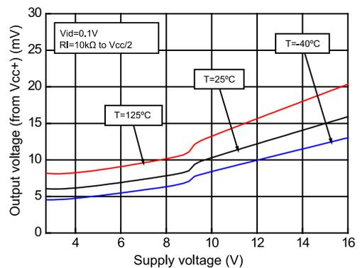
Figure 14: Output voltage vs. input voltage close to the rail at  $V_{CC} = 16\text{ V}$
