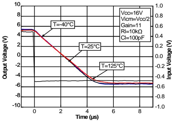
Figure 17: Positive slew rate at  $V_{CC} = 16\text{ V}$
