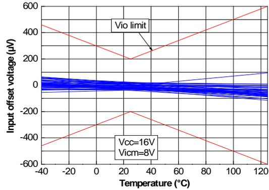
Figure 6: Input offset voltage drift population
