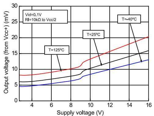
Figure 14: Output voltage vs. input voltage close to the rail at  $V_{CC} = 16$  V
