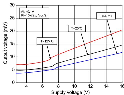
Figure 13: Output high voltage (drop from  $V_{CC+}$ ) vs. supply voltage
