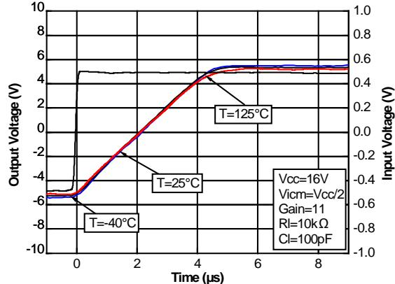
Figure 18: Response to a small input voltage step
