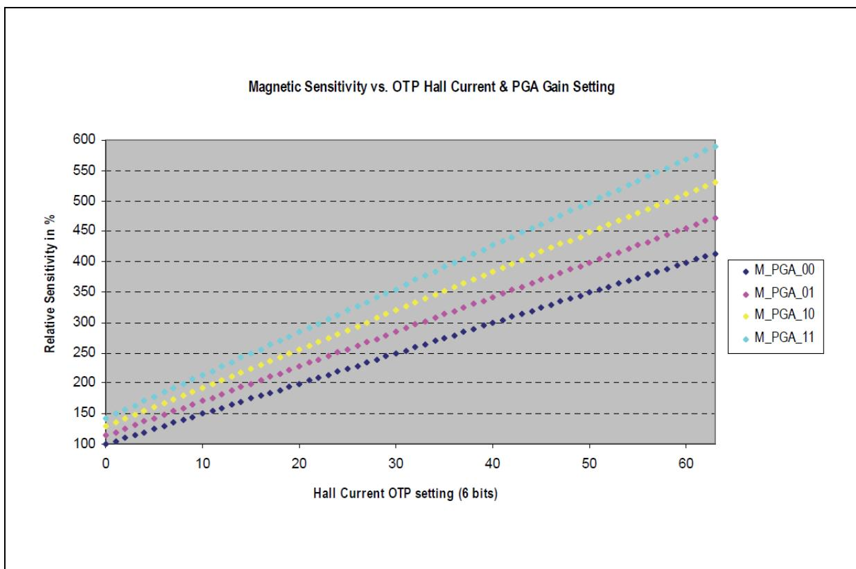
The amplitude of the output signal is programmable via sensitivity (6bit) and/or gain (2bit) settings (see [Figure 16](#)).
