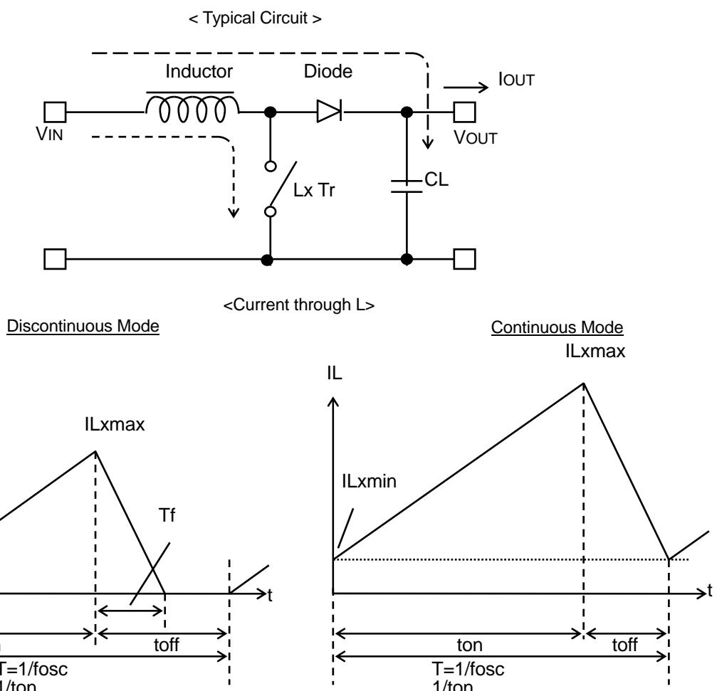
In PWM step-up switching regulator, there are two modes, the discontinuous mode and the continuous mode. These two modes depend upon the continuous characteristic of the inductor current.
