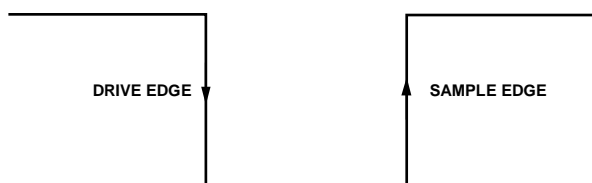
Figure 45. SPI Mode 3 SCLK Edges
