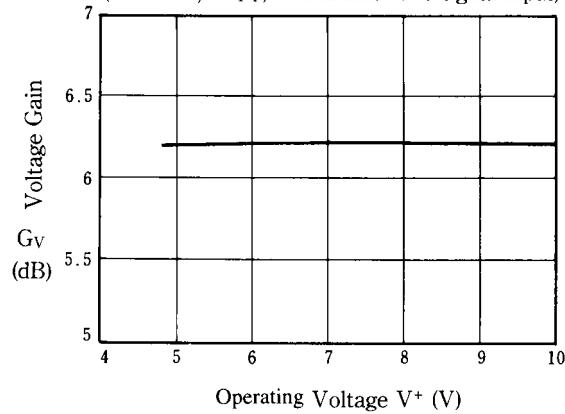
**Gain Frequency Characteristics vs. Operating Voltage**
