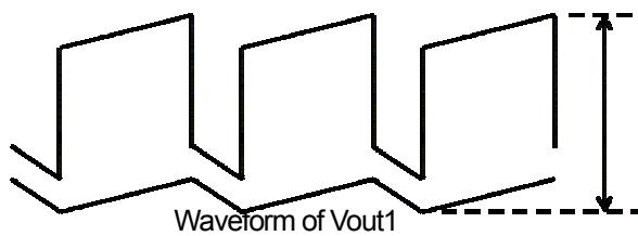
not using SAG correction circuit
