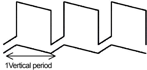
SAG correction circuit generates a low frequency component signal amplified to Vout terminal. Changes of the luminance signal will be low-frequency components, if you want to output a large signal luminance changes. Therefore, generate correction signal of change of a luminance signal to Vout pin. At this time, signal is over the dynamic range of Vout pin. This may cause a lack of sync signal, and waveform distortion.
