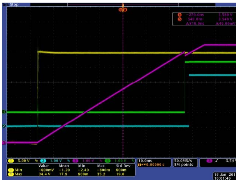
Figure 6. NCN5150 Startup Sequence
