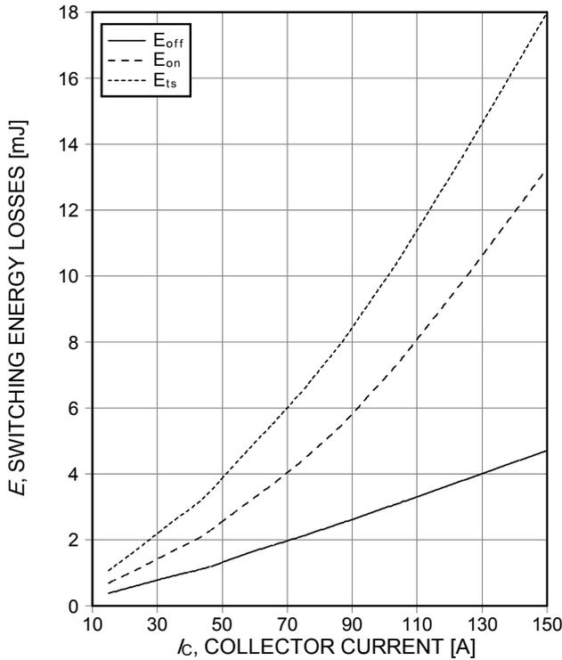
**Figure 13. Typical switching energy losses as a function of collector current**
