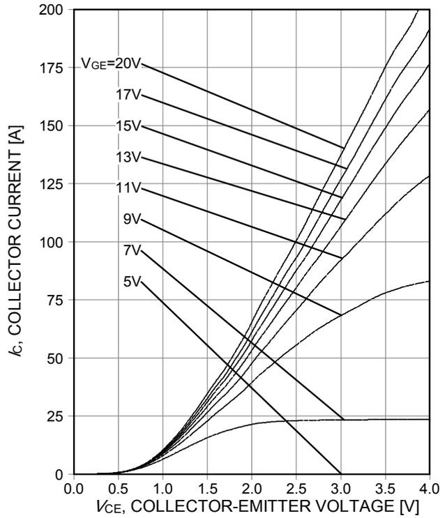
Figure 6. Typical output characteristic ( $T_j=175^\circ\text{C}$ )
