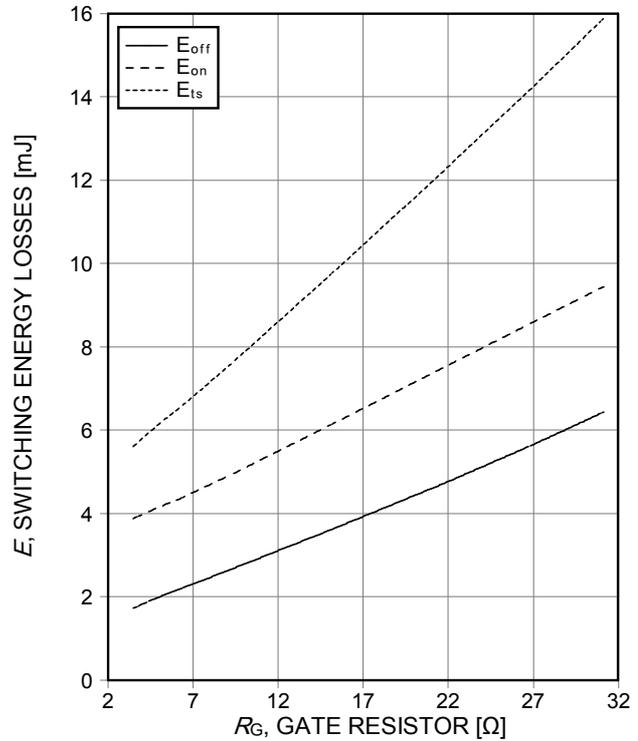
**Figure 14. Typical switching energy losses as a function of gate resistor**
