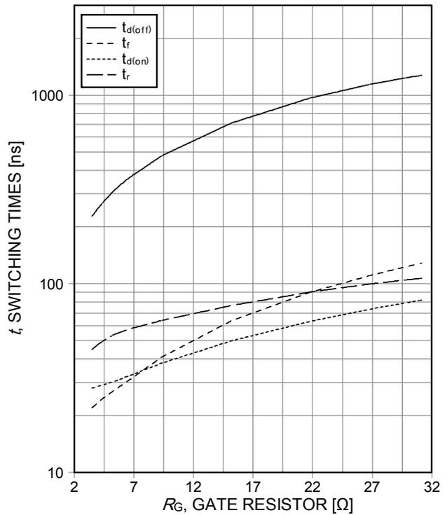
**Figure 10. Typical switching times as a function of gate resistor**
