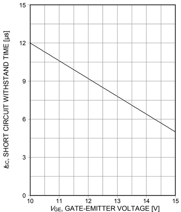
Figure 20. Short circuit withstand time as a function of gate-emitter voltage
