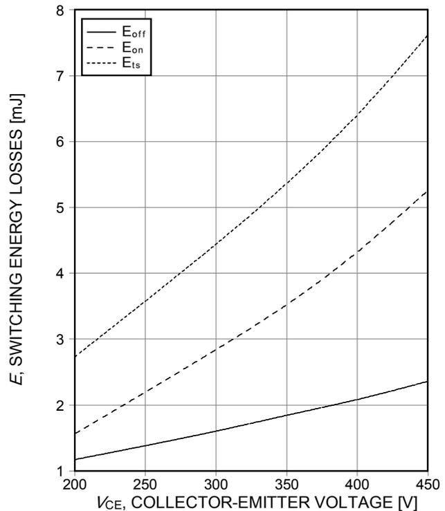
**Figure 16. Typical switching energy losses as a function of collector emitter voltage**
