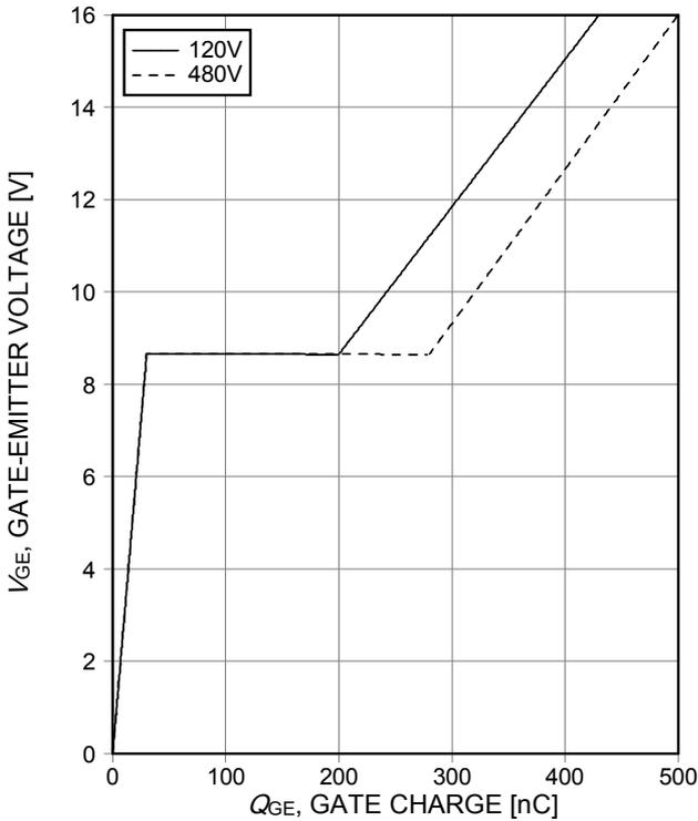
Figure 17. Typical gate charge
