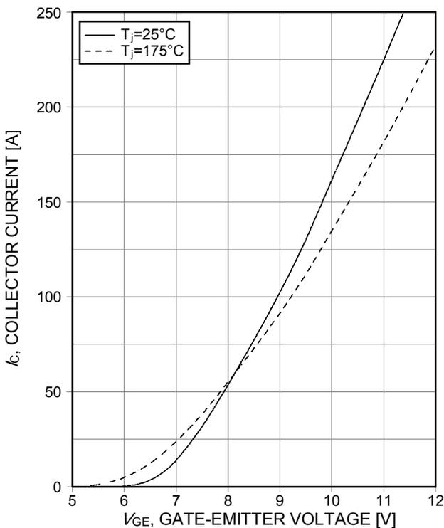
Figure 7. Typical transfer characteristic ( $V_{CE}=20\text{V}$ )
