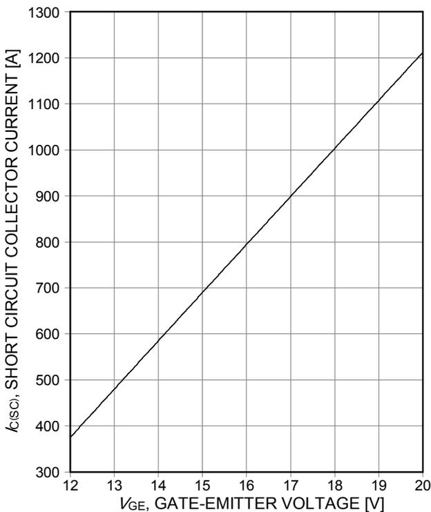
Figure 19. Typical short circuit collector current as a function of gate-emitter voltage
