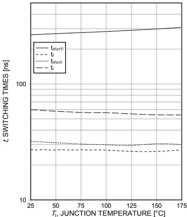
**Figure 11. Typical switching times as a function of junction temperature**
