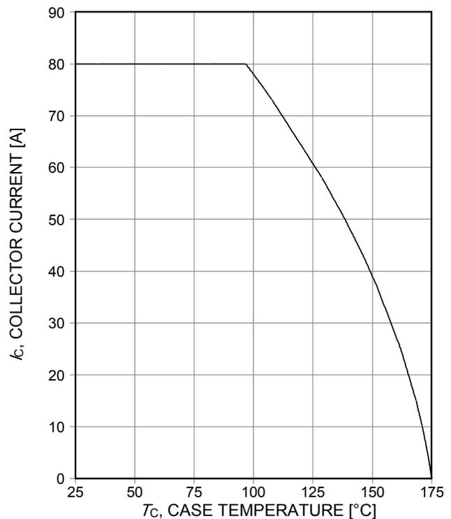
**Figure 4. Collector current as a function of case temperature**
