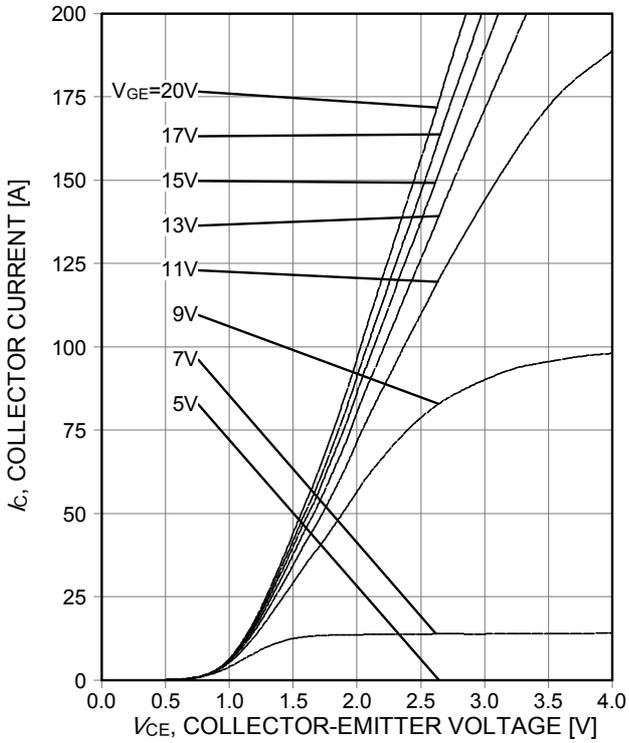
Figure 5. Typical output characteristic ( $T_j=25^\circ\text{C}$ )
