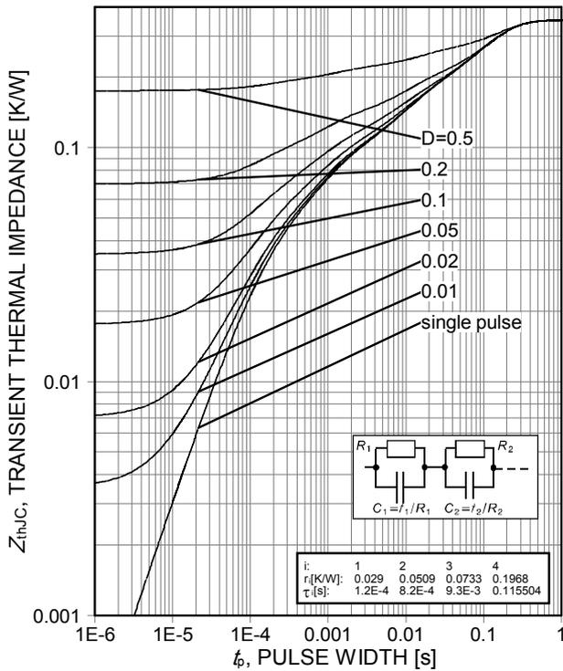
Figure 21. IGBT transient thermal impedance ( $D = t_p/T$ )
