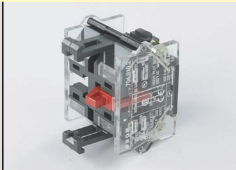
Contact block, screw terminal, slow-make with forced opening silver contacts
