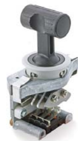
Lever switch, 2-5 positions, plug-in or screw terminals, aluminium bezel, silver contacts with positive opening, 33.5mm mounting
