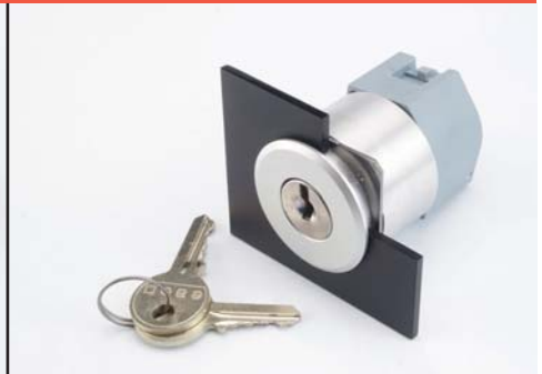
Keylock switch 2 position, flush mount, 30.5mm mounting
